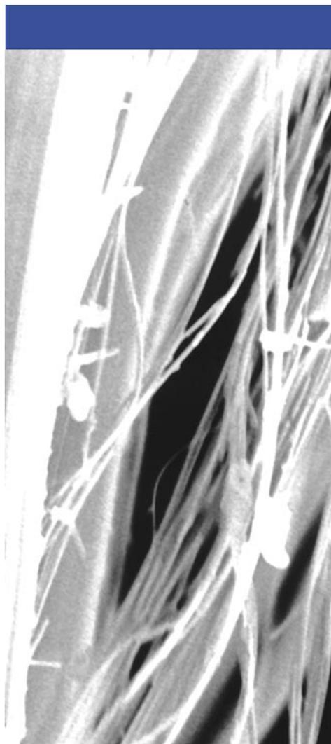
Magnification of Asbestos Fibers
